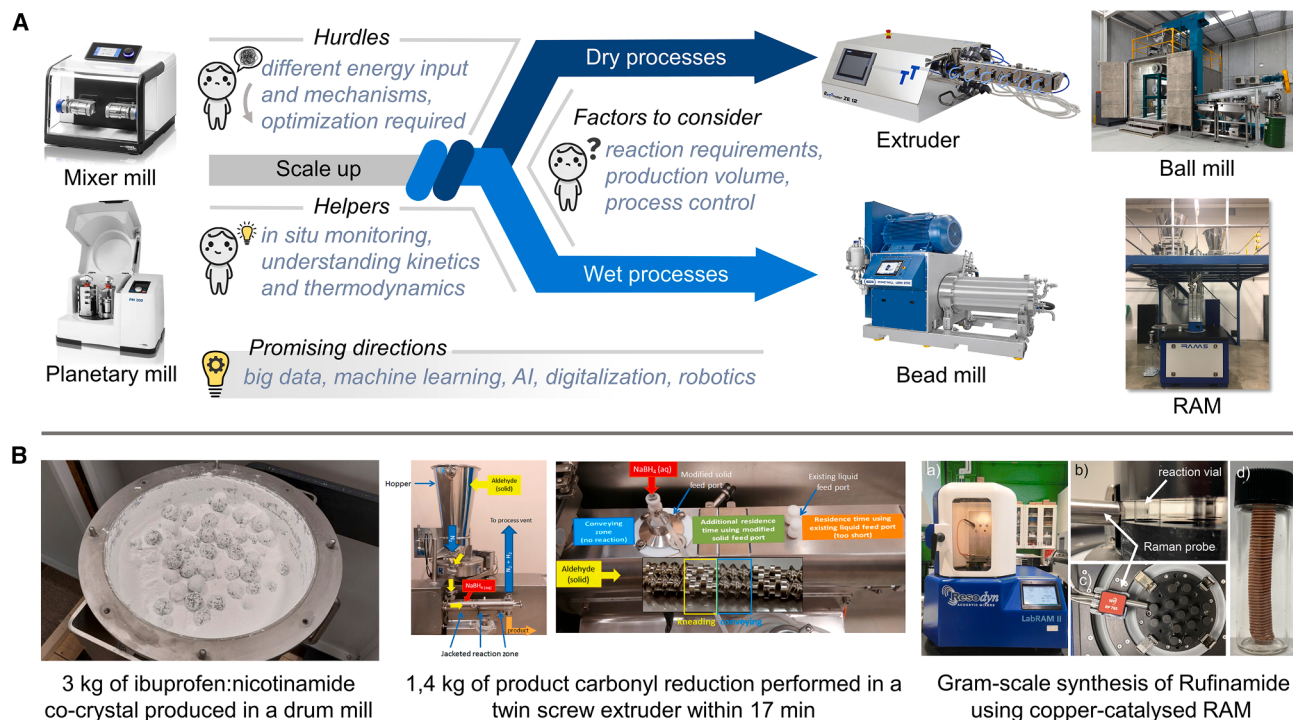
Figure 9. Continuous approaches for scaling up mechanochemical processes: TSE, ball milling, bead milling, and RAM
